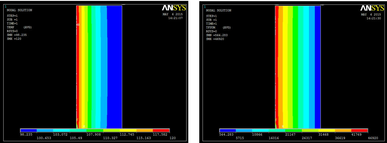
Figure 13. temperature distribution contours and Heat fluxes contours of fin P10.
