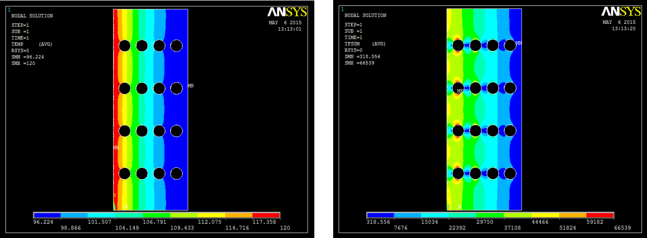
Figure 7. temperature distribution contours and Heat fluxes contours of fin P4.
