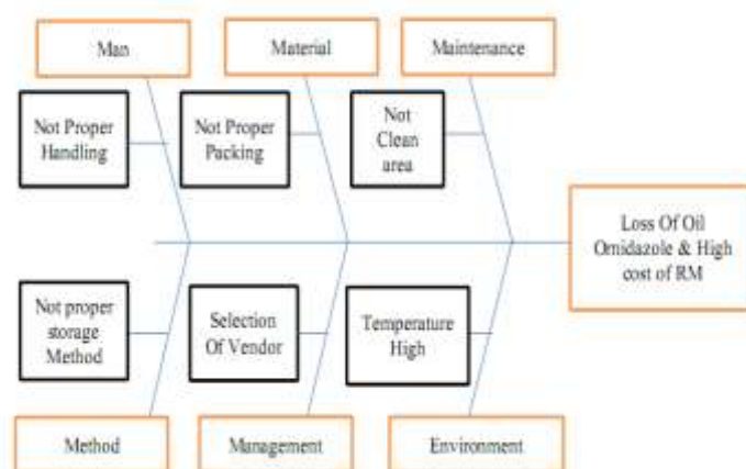
Figure 6. Fishbone diagram shows causes of raw material loss
