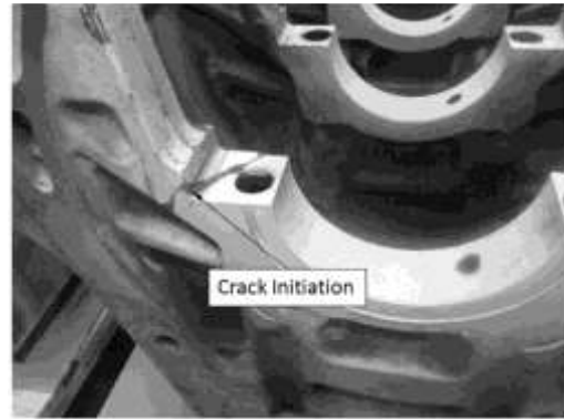
Figure 3: Crack at main bearing (flywheel side)
