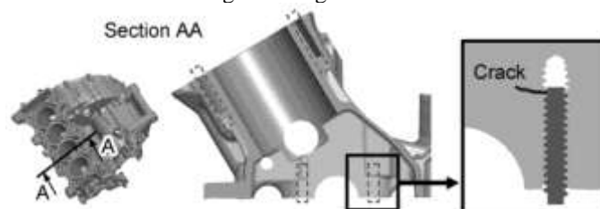
Figure 23: Location of starting point of fatigue fracture at internal thread
