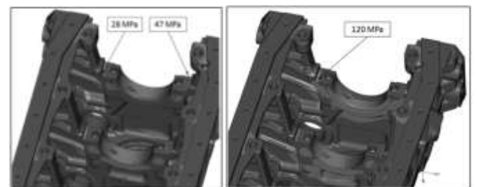
Figure 6: Maximum principle stress at main bearing for load case 3 and 4 respectively
