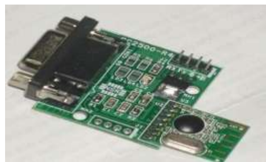
Figure 6. RF Transceiver module [7]
